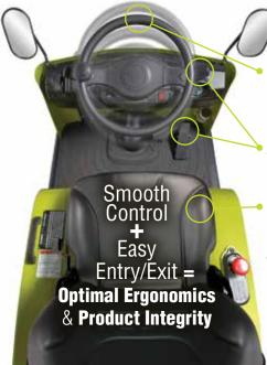
26° Tilt Steering Column maximizes operator's driving preferences.
