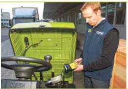
• The CLARK handset can be used for diagnostics and settings of up to 20 different performance parameters to match your requirements.
