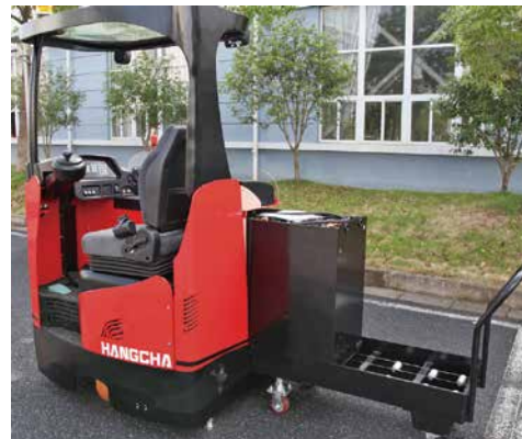
Standard configuration: Battery side roll-out + trolley(optional)
