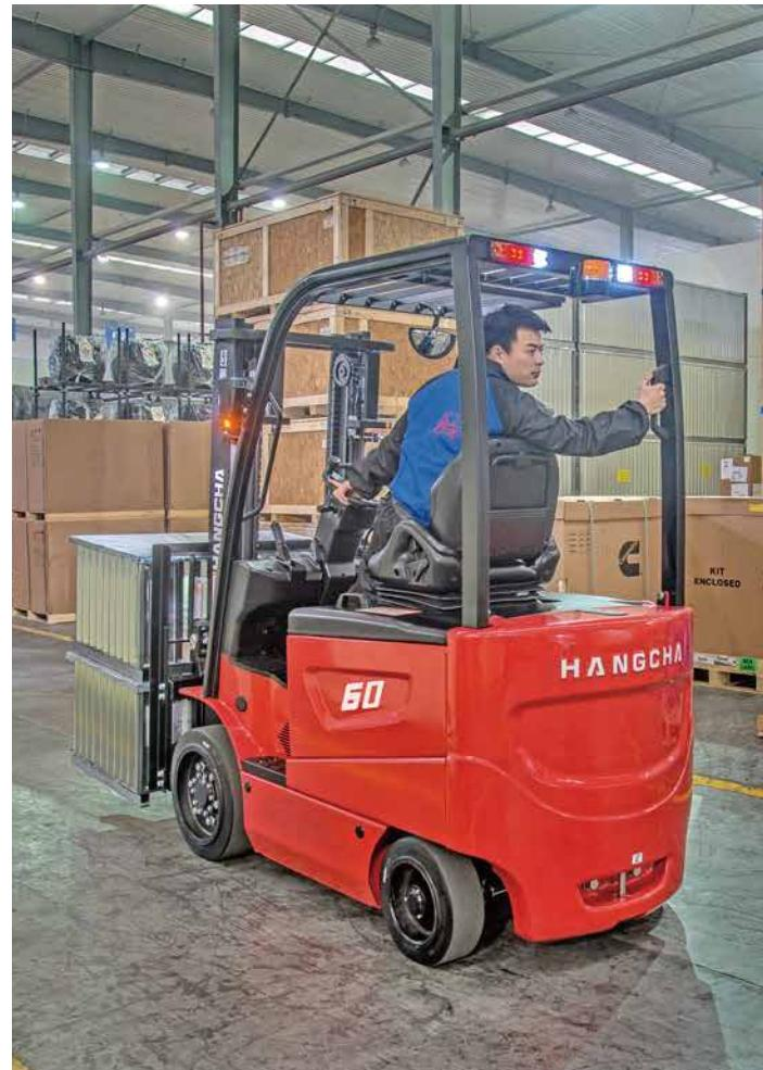
Rear handle with horn offers higher safety when the operator is reversing the truck.
