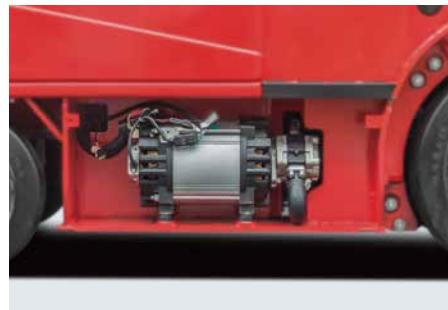
Innovative dual-door structure, with one door at left side and right side of the truck respectively, enables easy maintenance of oil pump motor, oil pump, and electric control of the truck, with good waterproof and dustproof performance.
