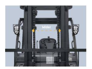
The new design mast provides broad forward visibility due to the distance between inside mast is increase 60mm.
