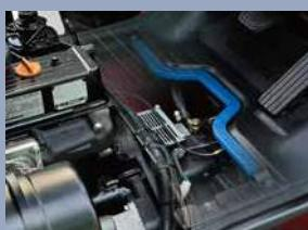
In addition to rubber damper between frames and steering axle, compound engine damper and full floating power train achieve flexible connection between frames and driving system, as a result, traveling vibrations and vibrations from the driving system are significantly reduced.
