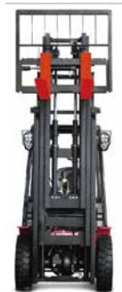
The developed front lifting cylinders with smaller outer diameter give the operator superior forward visibility.
