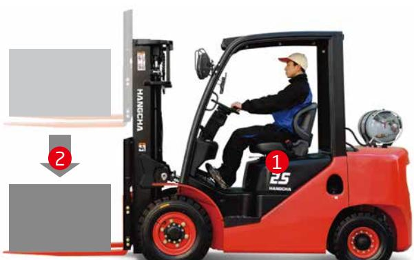
1. The operator presence sensing system incorporates lifting/tilting and traveling locking function. When the operator leaves the seat, the system automatically locks lifting / tilting and disables traveling to ensure safety.
