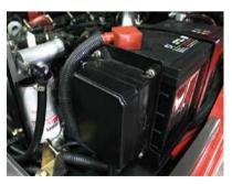
The new controller integrates all electrical components, features excellent durability for temperature, water and vibration for most demanding operation.
