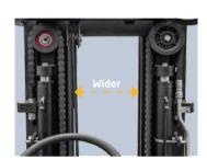
The developed front lifting cylinders with smaller outer diameter give the operator superior forward visibility.
