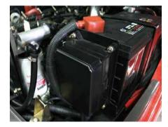
The new controller integrates all electrical components, features excellent durability for temperature, water and vibration for most demanding operation.
