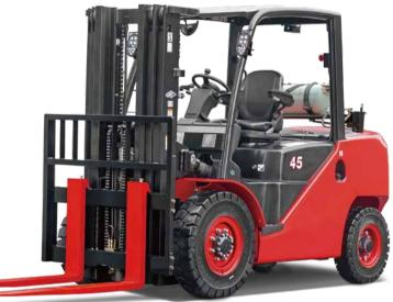
In developing the XF Series, comfort and ease of operation is carefully considered, for example, to improve vibration levels, compound engine damper and full floating power train are adopted. Comfortable operating environments for operator also contribute to increased productivity.
