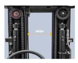
The developed front lifting cylinders with smaller outer diameter give the operator superior forward visibility.
