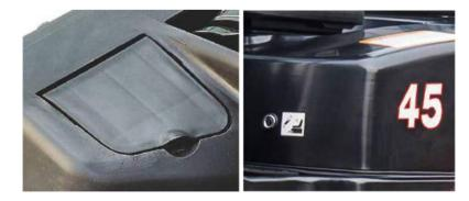
The cover on the Panel can be lifted up simply to check the brake fluid.
